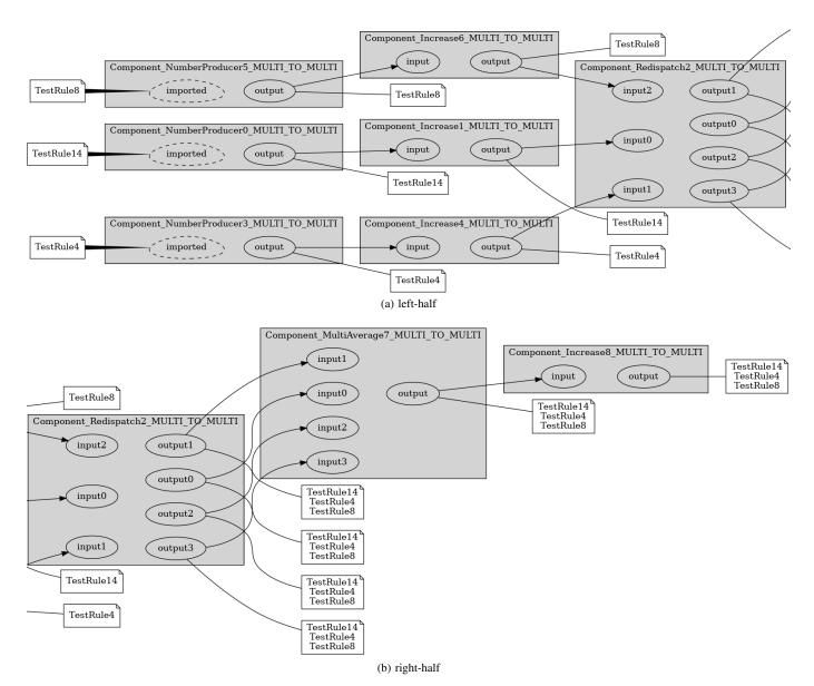
Figure 5: Reasoning result based on the provenance from executing the "redispatching" workflow (Fig. 4). Due to its width, the figure is split into two halves (sharing Component\_Redispatch2\_MULTI\_TO\_MULTI): subfigure (a) is the left-half; (b) is the right-half. In addition to Fig. 4: note-shapes are rules; lines (without arrows) connect the ports and the corresponding rules; black triangle arrows indicate *imported rules*; egg-shapes indicate virtual port; components are greyed.
