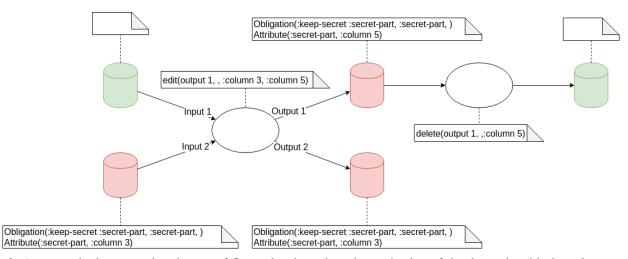
Figure 2: An example demonstrating the use of flow rules: here they show adaption of the data rule with the column number change. Ellipse for processes; cylinder for data; note-shape for rules; green for data without sensitivity; red for data with sensitivity; the flow rules here follow the default propagation (i.e. everything in to everything out).
